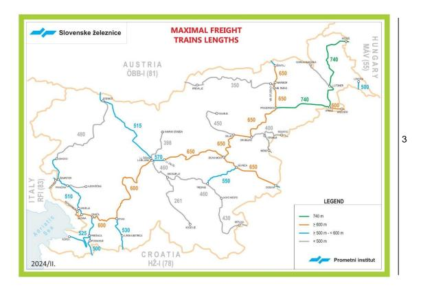
The maximum train length permitted on the PRI is 430m for passenger trains and 740m for freight trains. Freight train lengths may be additionally limited at stations with short tracks, as shown in the table below.
