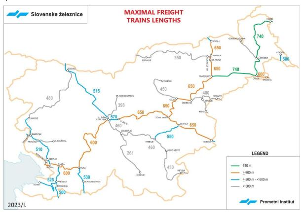
The maximum train length permitted on the PRI is 430m for passenger trains and 740m for freight trains. Freight train lengths may be additionally limited at stations with short tracks, as shown in the table below.
