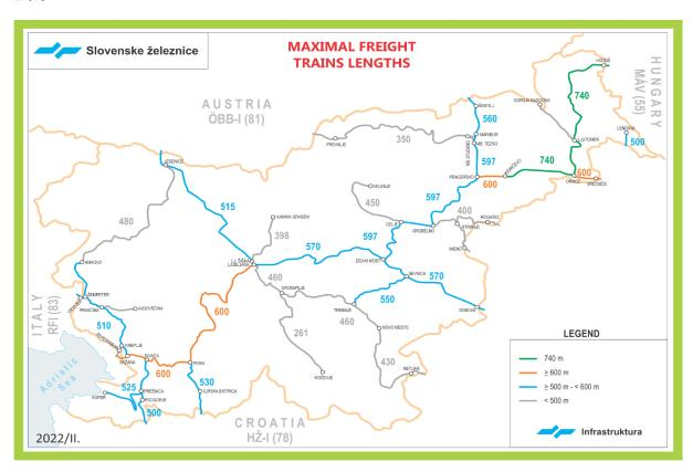
The maximum length at which a train may operate on a route section of Slovenian rail network is determined by the usable length of station tracks, which is taken into account in capacity allocation and optimisation.
