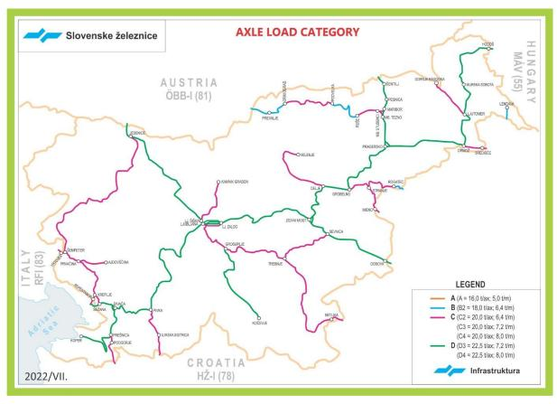
The table under Chapter 2.2 provides a broad indication of line categories on the PRI by axle and meter load. Details about the weight limits on a particular route section can be found in the map below and in Annex 2A.
